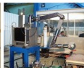
Hydraulic manipulator for dismantling operations
